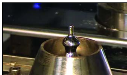
Nozzles with enhanced capability now include a production 1.5mm nozzle.
